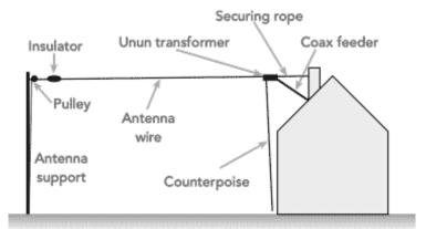
Resonance: Random wire antennas are not resonant, meaning they have a high standing wave ratio (SWR) on most frequencies. They do not have a specific length that corresponds to a half or quarter wavelength.
